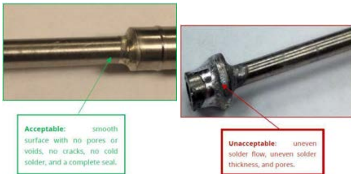
Figure 16-3: Failed lead-free solder trial
