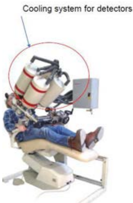
Figure 4-6: Lung counter with a cooling system
