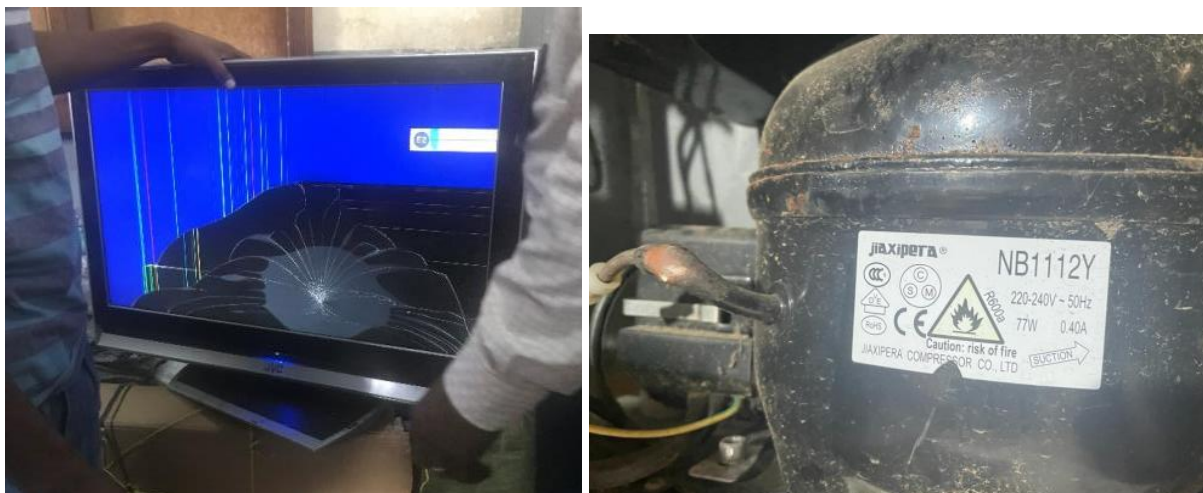
Figure 4 Screen regarded as e-waste after visual inspection (left), identification of refrigerant (right)
